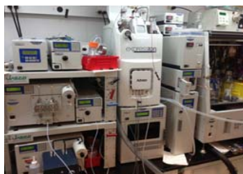
JASCO Preparative SFC system with fraction collection and Advion expression
