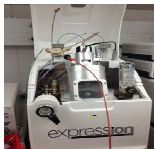
ZDV splitting Tee pre CMS, splits in the LCMS make-up solvent for ionization and sample stream from 2nd ZDV Tee PEEKSil line.
