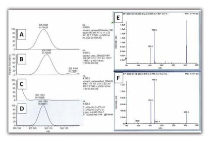
(A) HRMS of the protonated molecule region at m/z 305 for diazinon extracted from the spinach leaf surface.
