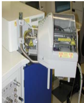
Figure 1. Advion NanoMate 100 automated nano-electrospray system installed on a Micromass Q-TOF 1 mass spectrometer
