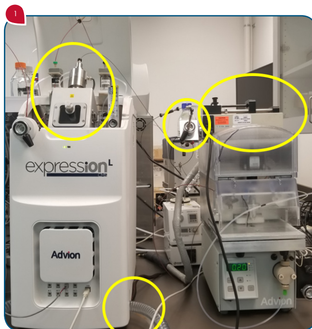
Figure 1: The CMS with standard APCI source at 4 L/min Nitrogen gas flow, additional source exhaust to house vacuum and FIA sample introduction using a syringe pump at 30 µL/min, a 10 µL loop and all PEEKSil tubing to the source.
