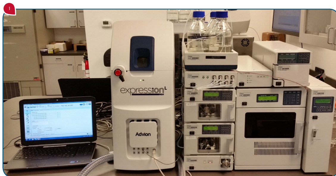
Figure 1: UHPLC/CMS set up for the detection and quantification of amino acids in complex mixtures utilizing a JASCO X-LC system, an Imtakt Corporation Intrada Amino Acid HPLC column, and the Advion expression + CMS.
