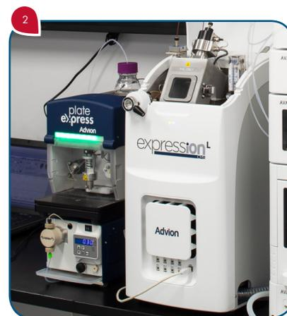
**Figure 2:** Instrument setup with the CMS and Plate Express for TLC/CMS.
