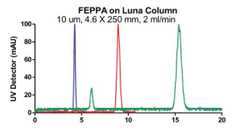
HPLC chromatograms of FEPPA, using a Luna C18 ODS (4.6 X 250 mm, 10  $\mu$ m) and 3 different ethanol and 0.1 M ammonium acetate based mobile phases. (60% Ethanol, Blue line), (40%, Ethanol Red line) and (20% Ethanol, Green line).
