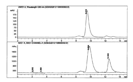
Confidential antibody, DTPA chelator. 4M reactor. Stop flow reaction reagents ( 15  $\mu$ l Antibody and 15 $\mu$ l isotope ) held in loop for 35 minutes at 45°C .
