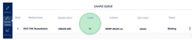
Continuous operation is achieved by assigning the number of "Cycles" in the sample queue in the chromatography software. The number of cycles is the number of loads of distillate you wish to process in a shift. At the end of each 48 minute method, a new distillate load will take place in the next cycle.
