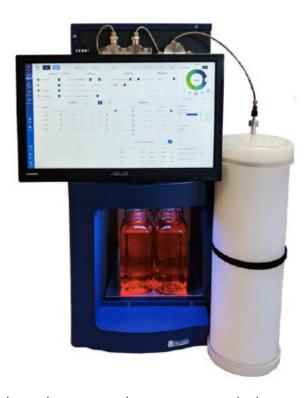
Pilot and process scale instruments are built to specification and utilize hydraulic piston columns with inner diameters from 20 cm to 100 cm.
